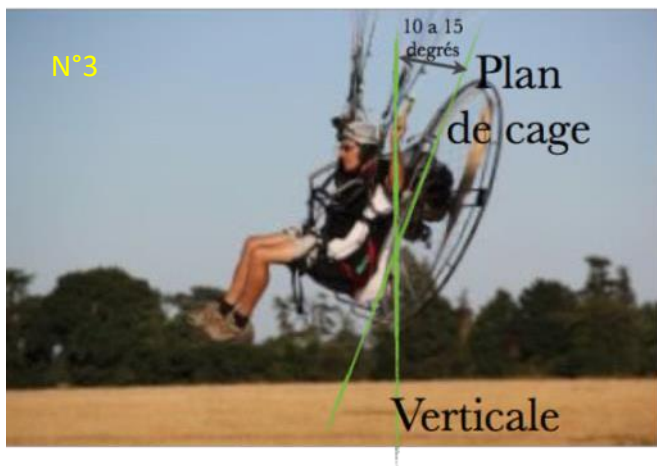
Propeller plan to be checked on the gantry before starting a flight
