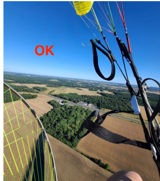
Brake control on its magnet OK
