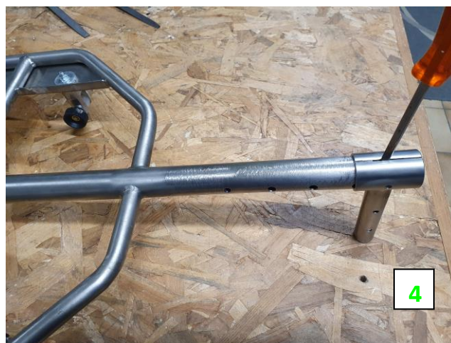
Support spacing for interlocking on the central tube
