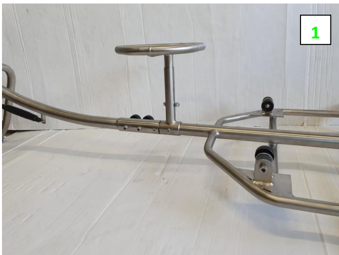
Cutout of the base of the seat support tube with an incision lengthwise
