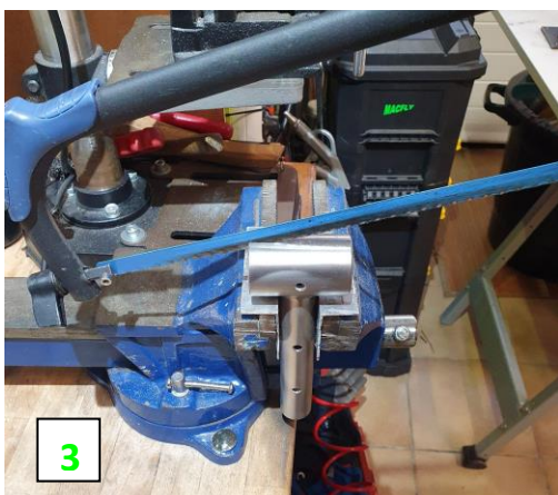
Cutout of the base of the seat support tube with an incision lengthwise
