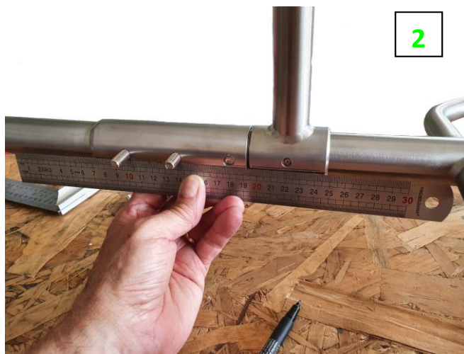
Support spacing for interlocking on the central tube
